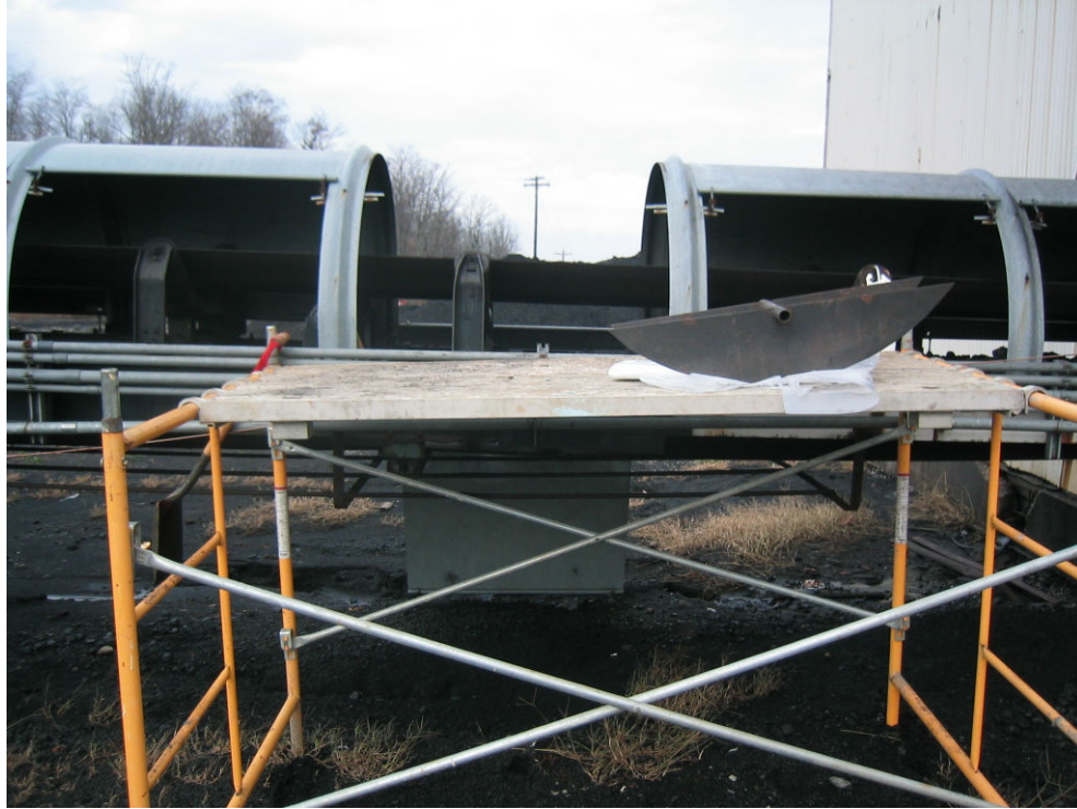
Figure 2. Photograph of the stopped belt sample collection site and cutter
